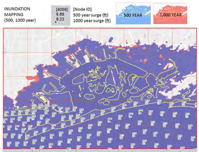
**Figure 3.8:** Sample Inundation Model Results Using ADCIRC model
