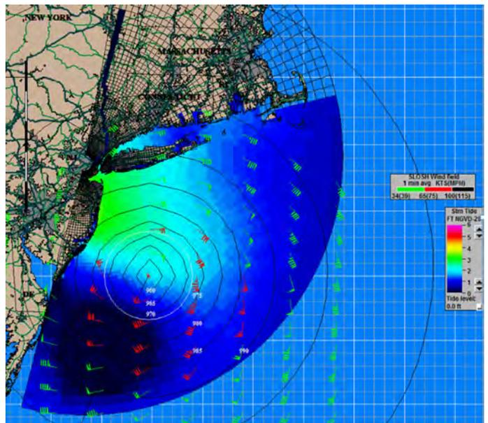
**Figure 3.9:** Sample SLOSH Simulation Using the NY3 Basin Displaying Wind Field and Tidal Data
